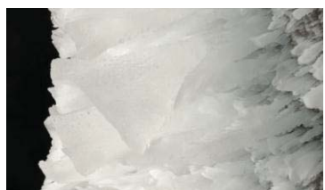
Figure 19. Ice shape for 45° swept wing. Icing conditions: airspeed 103 m/s; icing time 20 minutes; liquid water content, 0.45 g/m 3 ; static temperature, 261 K, static pressure, 94463 Pa; MVD, 32 μm.
