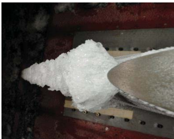
Figure 12. - Concluded. Ice shape comparisons for 45° swept wing. Icing conditions: airspeed 45 m/s; icing time 20 minutes; liquid water content, 1.5 g/m 3 ; static pressure, 99981 Pa; MVD, 15 μm.
