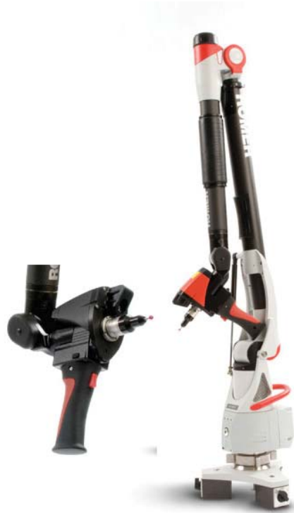
Figure 4 Romer scanner used for this study.
