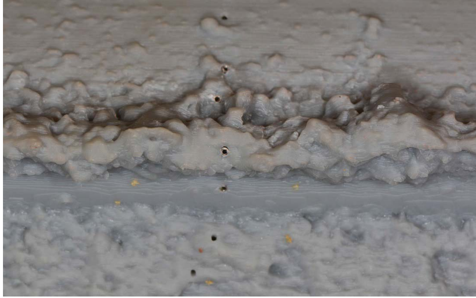
Figure 19 Pressure taps on artificial RPM ice shape.
