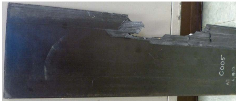
Figure 14. C005 Impact Damage
