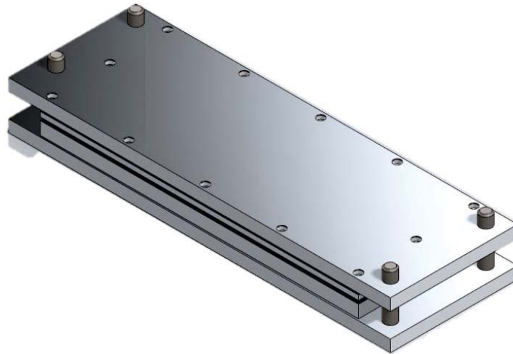
Figure 9. 3-D model of mated die mold
