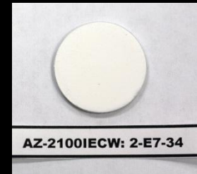
AZ Tek AZ-2100 thermal control coating: data from this and other samples led to it being chosen for Curiosity's radiator
