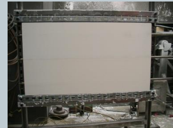
PS-16 thermal control coating on test radiator
