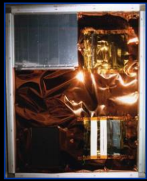
AO erosion of Kapton blanket
