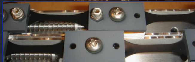
Stressed (left) and unstressed (right) samples
