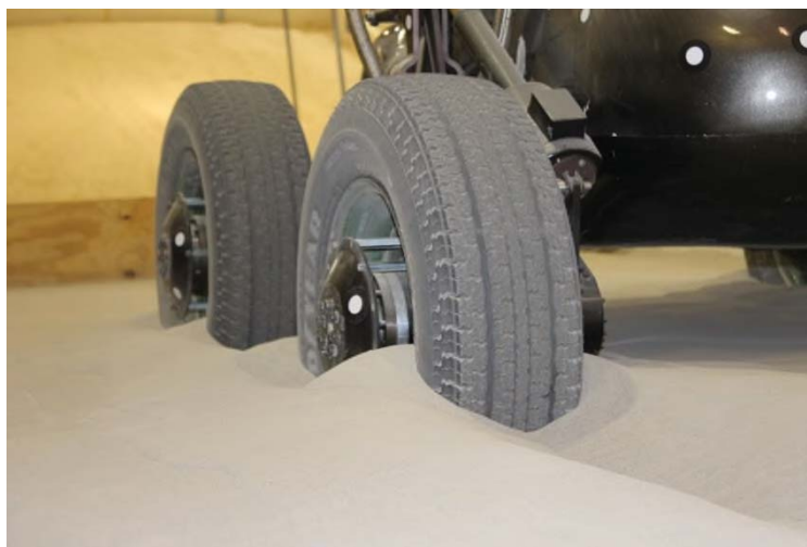
Figure 6.—Pneumatic rubber tires buried in Fillite.
