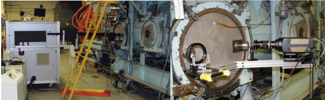
Figure 2. Photographs of the NO PLIF system. Set up adjacent to the AHSTF showing the mobile PLIF cart and facility (left) and detail of camera setup (right). The configuration shown was used in the first set of experiments (Configuration 1 in Table 1).
