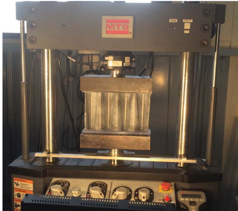
Figure 13. Static crush specimen
