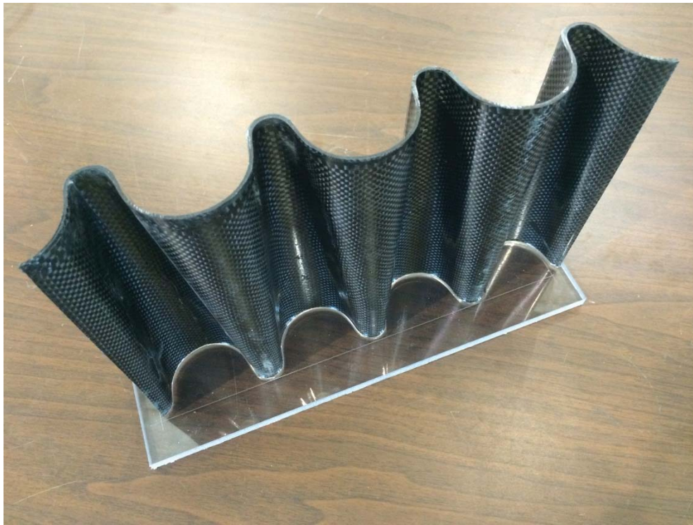
Figure 5. Completed conusoidal specimen
