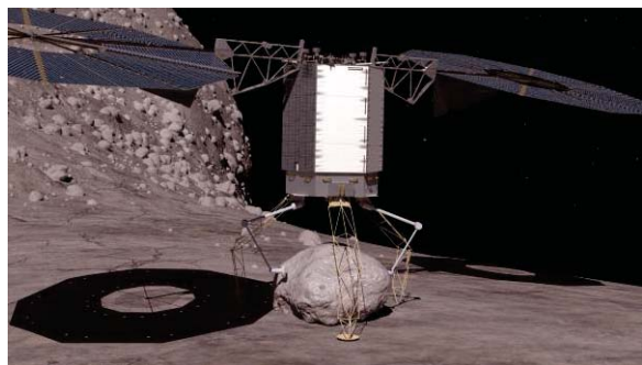
Fig. 5: ARM robotic boulder capture option (Credit: NASA/AMA, Inc.).
