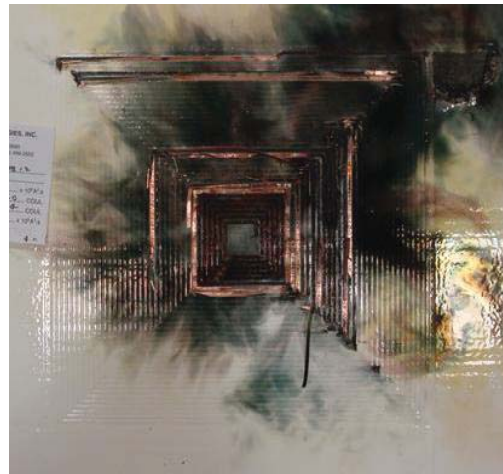
(a) Backside IR thermal image at 4 sec after strike. (b) Post strike photograph. Figure 9.16. Data of a 9" SansEC Sensor of FRC.
