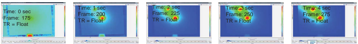
Panel backside IR image at sequential times. Note image has been flipped to provide a top side view.
