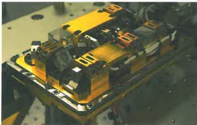
MLA Laser Transmitter – derivative of GLAS laser MOPA design, 8Hz, 20 mJ Detector – same as GLAS, SiAPD
