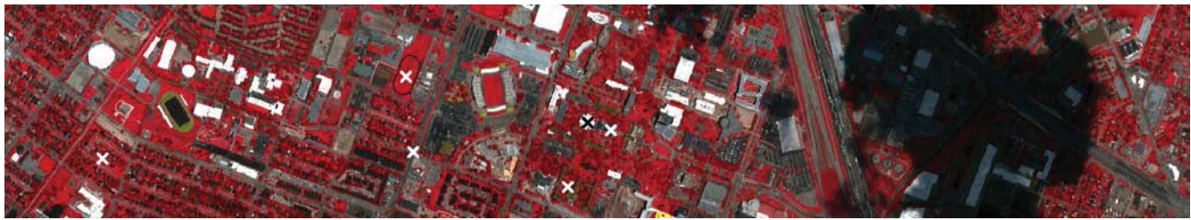
Fig. 7. False-color composite of the University of Houston dataset obtained from hyperspectral data (RGB: bands 105, 61, and 40).
