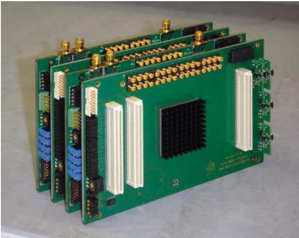
Fig. 1 Stack of DBBC3 boards for dual polarization.
