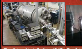
The Solar Wind Facility (SWF) exposes SPC to a range of ion and electron distribution energies.
