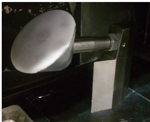
Fig. 2 Orion MPCV model at 52^\circ angle of attack configuration with naphthalene heat shield installed in the Mach 5 wind tunnel facility at The University of Texas at Austin.
