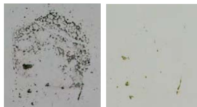
Fig. 2b. Droplet from 2a after UV ozone (left) and after UPW (right).
