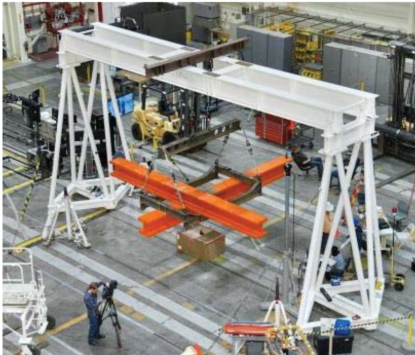
Figure 6. The iron bird undergoing I_{zz} pendulum testing.
