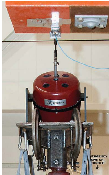
Figure 8. An MB Dynamics (Cleveland, Ohio) shaker.
