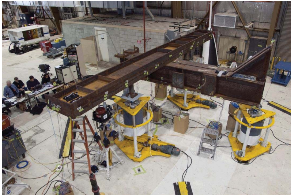
Figure 2. The initial iron bird test article undergoing DIM testing.
