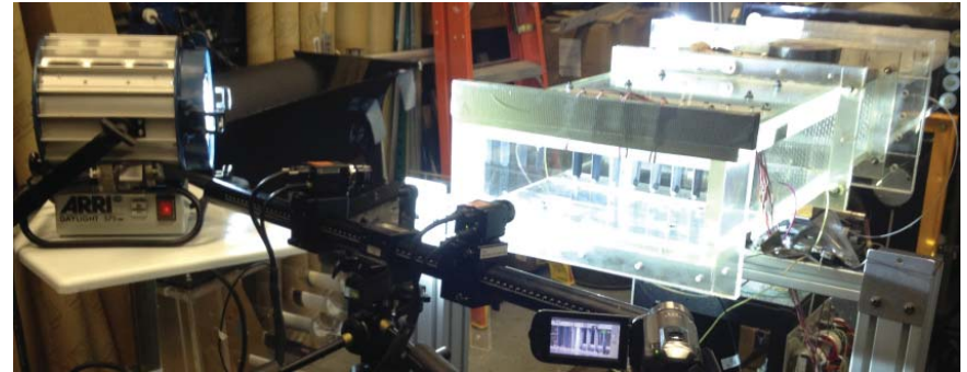
Test rig with Digital Image Correlation system for measurement of vane deformation
