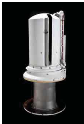
Fig. 6: A back-up camera identical to the original photodiode camera of the Viking Lander mission to mars: 40.64cm tall x 21.59cm wide, 7.3kg. 29
