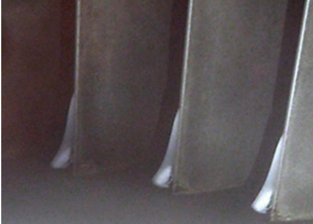
Figure 34. Ice accretion forming on bottom leading edge of LPC IGV during anti-ice off cloud on conditions.
