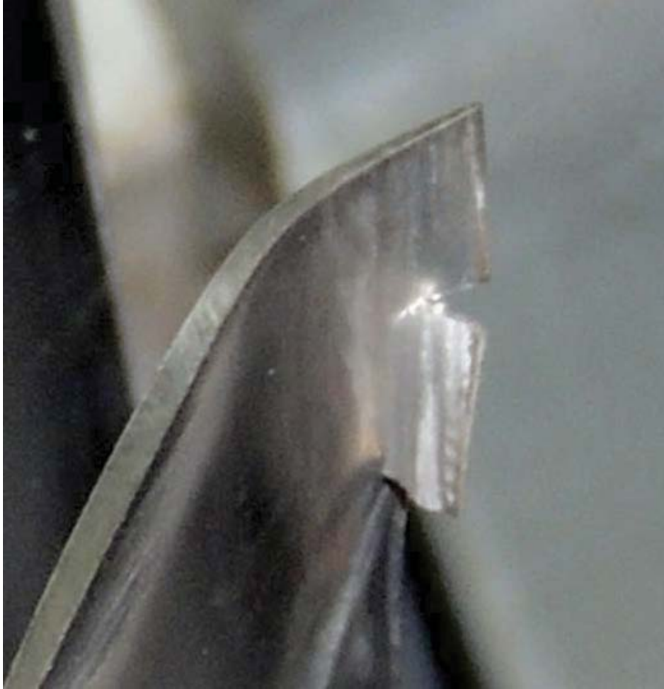
Figure 36. HPC Rotor 1 mechanical damage.
