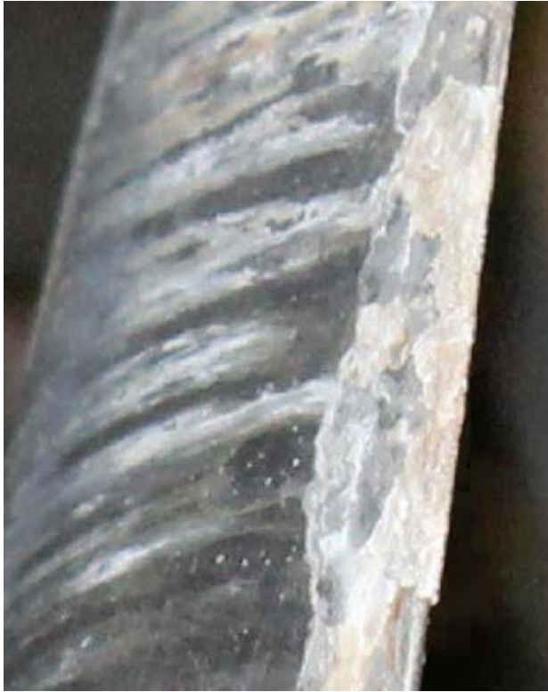
Figure 32. Mineral deposits on LF01 engine core flow path hardware.
