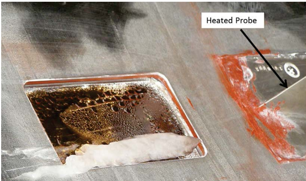
Figure 37. Ice mass accreting to side wall downstream of heated pitot probe.
