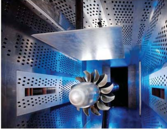
Figure 5. Model scale F31/A31 blade set installed in the NASA 8-foot x 6-foot high-speed wind tunnel. The plate shown suspended above the rotor has embedded Kulites that were used for nearfield acoustic measurements, which were used for assessing the acoustic predictions in this paper.
