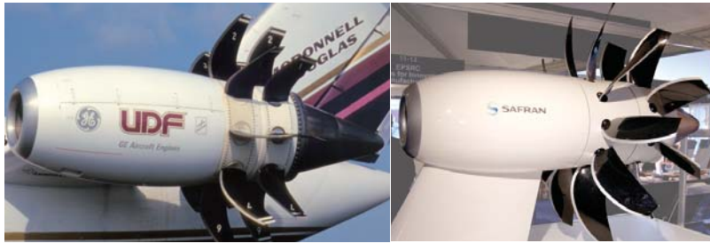
Figure 1. On the left GE36-UDF propfan demonstrator engine installed on the MD-81 test bed aircraft in 1987 is shown. On the right is a model of a modern contra-rotating open rotor engine design from Snecma. Whereas the front and aft rotor blade counts were same on the UDF demonstrator engine (8 x 8), the modern CROR engine designs feature unequal blade counts (typically, 12 x 10).
