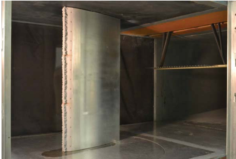
Figure 1. NACA 23012 airfoil model installed in the University of Illinois wind-tunnel test section with artificial ice shape installed on leading edge.
