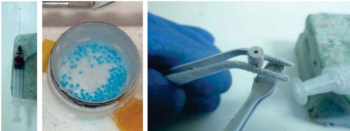
Figure 1. Photographs of syringe to create 500 \mu\text{m} water drops, 3,000 \mu\text{m} water drops frozen in LN2 and frozen droplet placed into sabot bullet.
