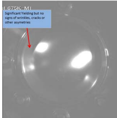
Figure 14 - AI 2024 Symmetrical Yielding Prior to Rupture (DC Test 040, AI 2024 0.020")
