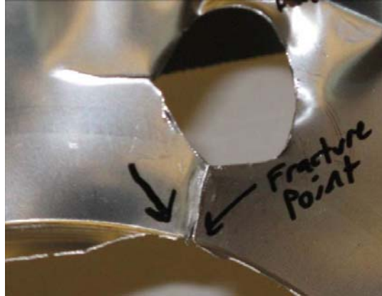
Figure 16 - Bolt Hole Tear linked to Point Failure (DC Test 063, 300 SS 0.015")
