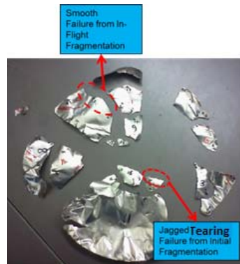
Figure 19 - Reconstructed Sample with Flower Petals shown (Test 028, 300 SS 0.004")
