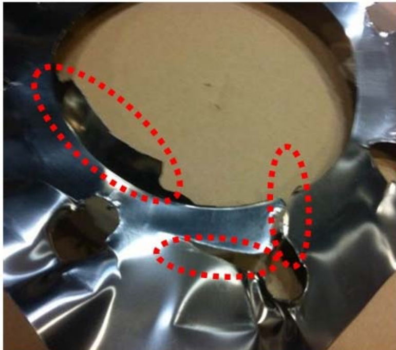
Figure 5 – Three common cracks on a sample remainder (DC Test 053, 300 SS 0.015”)
