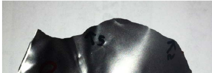
Figure 21 - Smooth Failure Characteristics (Highlighted from Test 028)
