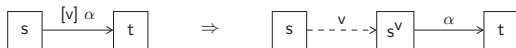
Figure 4: Transition mapping for HVM expansion. The transition from the HVM (on the left) induces two transitions in the expanded HMI-LTS (on the right).
