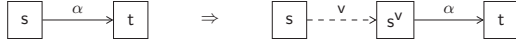
Figure 3: Transition mapping for HVS to HMI-LTS translation for non- \tau transitions. The transition from the original system model (on the left) induces two transitions in the expanded system model (on the right), where v = \mathcal{O}(s) .
