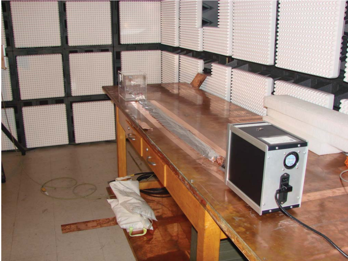
Figure D.3-11: RE02 Typical Antenna Setup, with Shielding
