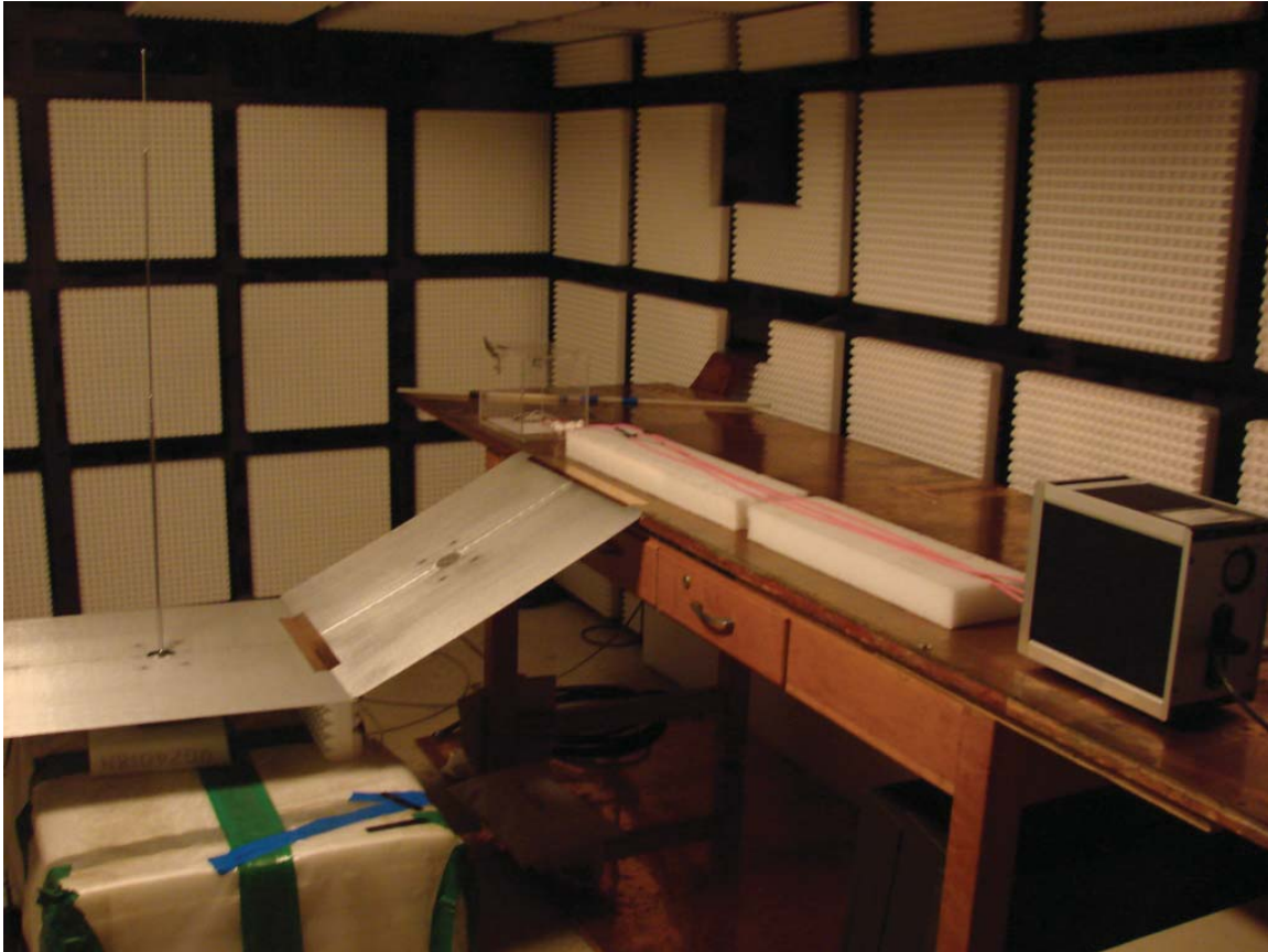
Figure D.3-8: RE02 Typical Active Rod Antenna Setup
