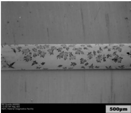
FIGURE 1 – an SEM image of a ZBLAN fiber processed in unit gravity. Clearly visible crystals were formed in the bulk of the fiber. These crystals significantly increase signal attenuation.
