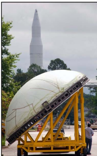
Ares I Upper Stage 5.5m diameter Pressurized Structure
