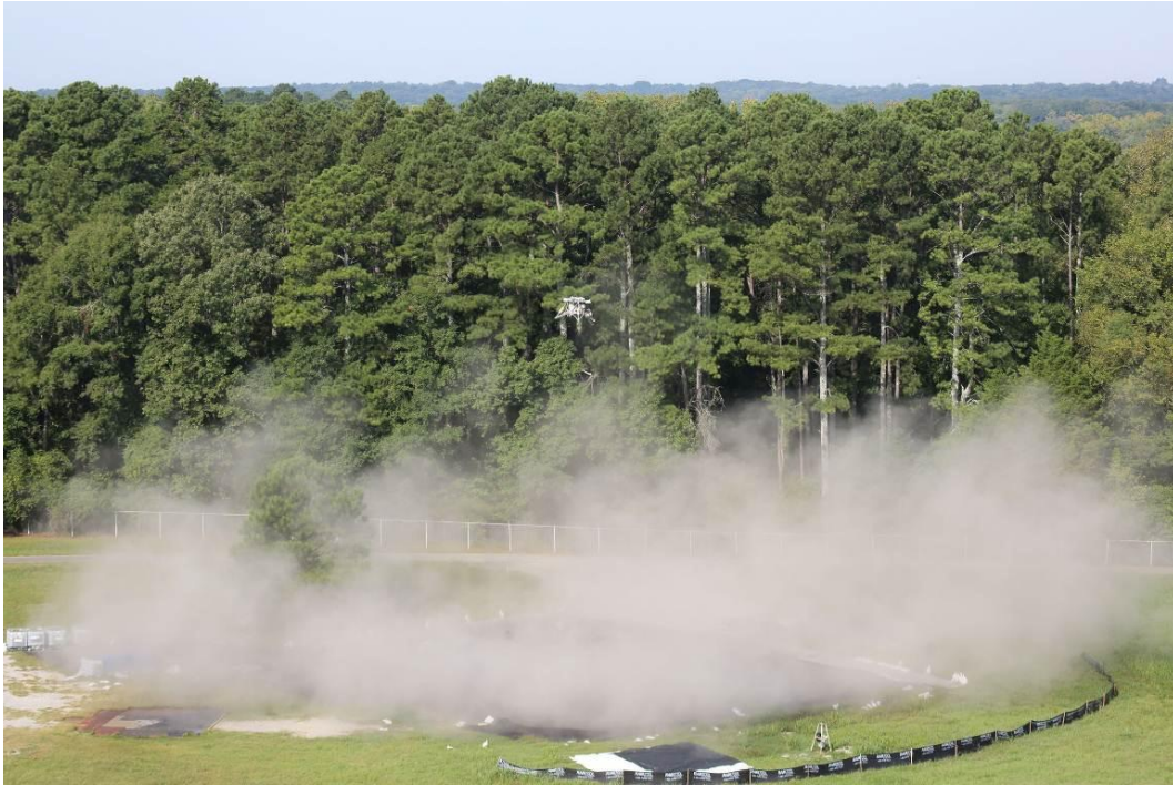
Figure 8. Large amount of dust generated by the plume from the Mighty Eagle on hazard avoidance as it traverses the terrain field at an altitude of 20 meters. Photo extracted from a video camera mounted on a quad-copter.
