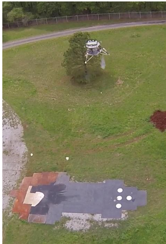
Figure 3. Mighty Eagle above the AR&C target in the West Test Area of MSFC. Photo extracted from a video camera mounted on a quad-copter.
