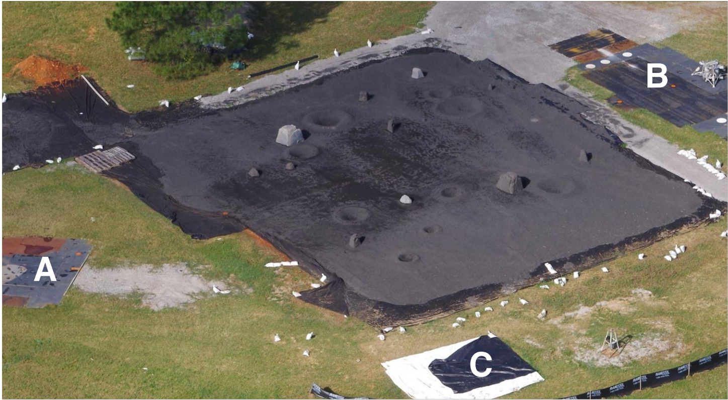
Figure 6. The MSFC Lunar Surface Terrain field. There are 9 craters and 11 boulders. A: steel plates for launch. B: steel plates for landing, with lander. C: folded infield tarp used to cover terrain field when not in use.
