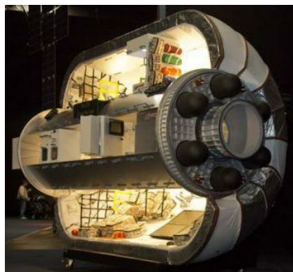
One example of an inflatable habitat, the proposed Bigelow Aerospace BA-330. Image credit: AP
