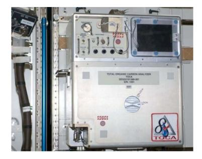
TOCA (total organic carbon analyzer) – measures total organic carbon concentrations in ISS water using IR
