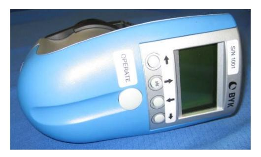
CWQMK (colorimetric water quality monitoring kit) – measures biocide levels (Ag,  $I_2$ /total lodine) in water using absorbance
