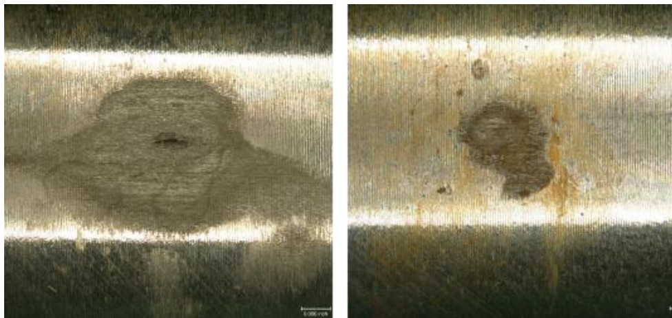
Figure 7. Pitting and corrosion on the external surfaces of the ALCLR housings.
