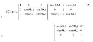
Once the attitude is updated, the attitude is used to help remove the affects of gravity  $g^E$  as well as centripetla and Coriolis acceleration due to the Earth's rotation. The updated  $\Delta \overline{v}_{EB}^{\ B}$  is defined in Eq. 16. In this case the instantaneous Earth gravity is given as  $g^E$  in the ECEF frame, and the notation  $[\omega_{IE}^{\ E} \times]$  represents the cross product matrix representation of the vector  $\omega_{IE}^{\ E}$  as shown in Eq. 17.
