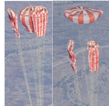
Figure 7. CDT-3-11 Main Skipping then Release.
