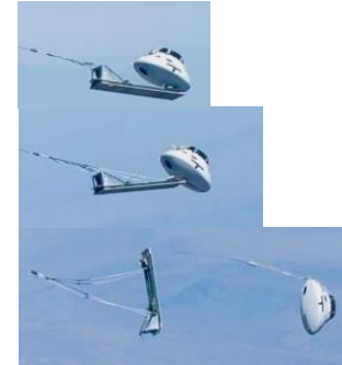
Figure 11. CDT-3-14 Apex Forward PTV Separation.
