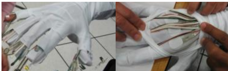
Figure 12: Glove wire guides and covers on fingers (left) and back of hand (right)
