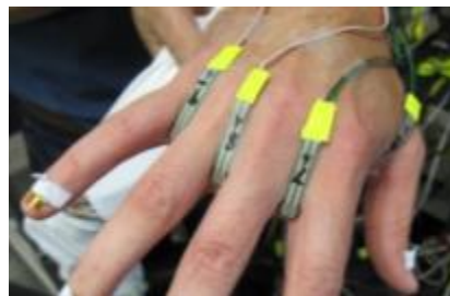
Figure 14: Small FSR finger crotch sensors beneath the base layer of the sensor glove
