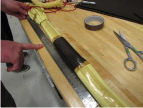
Photo 60. Test 11 setup (Short Teflon middle sleeve).
