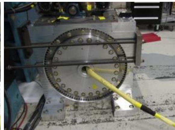
Photo 49. Test 7 setup (taped sleeves).
