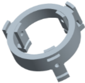
Figure 2. CAD model of edge radius fixture with turntable attachments.
