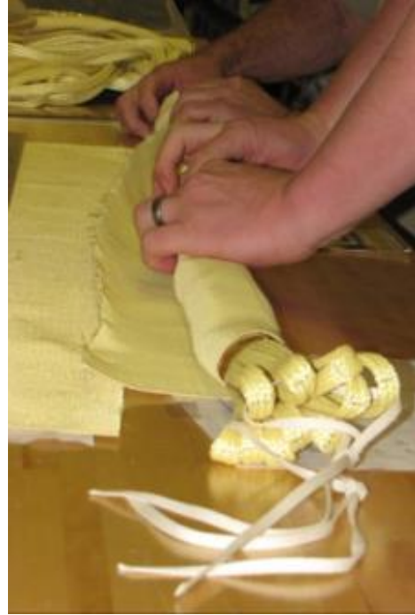
Photo 17. Riser sample being wrapped in Kevlar.
