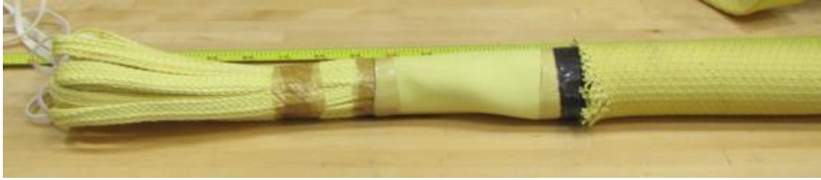
Photo 21. Riser sample with protective textile cover.
