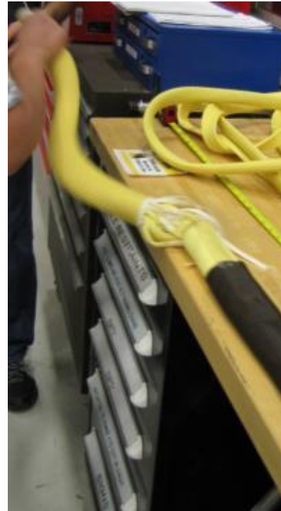
Photo 20. Riser sample being inserted into tubular Kevlar outer sleeve.
