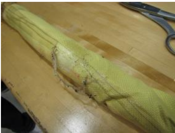
Photo 36. Test 1 effects (inner Kevlar sleeve).
