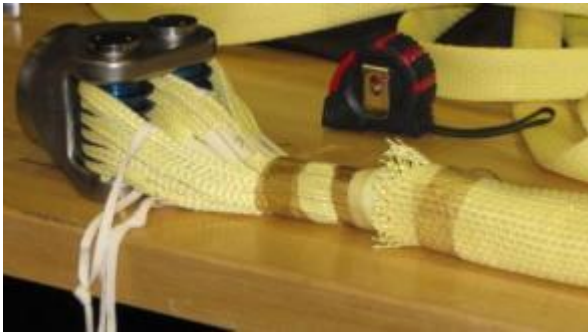
Photo 23. Riser sample with hardware interface “knuckle” attached (abrasion fixture end).
