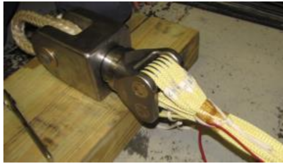
Photo 24. Riser sample with hardware interface “knuckle” attached (tensioned end).
