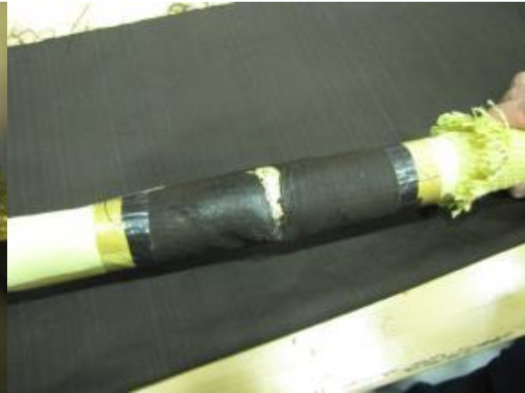
Photo 63. Test 11 results (middle sleeve).
