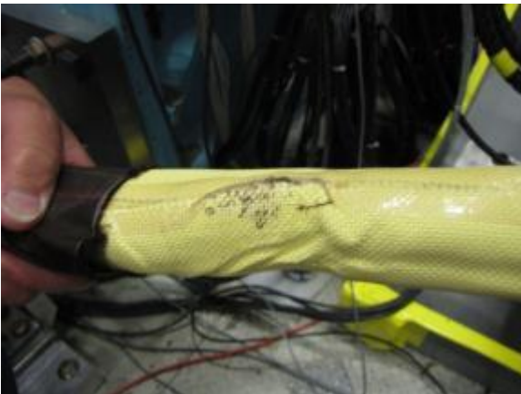
Photo 44. Test 2 effects (inner Kevlar sleeve).
