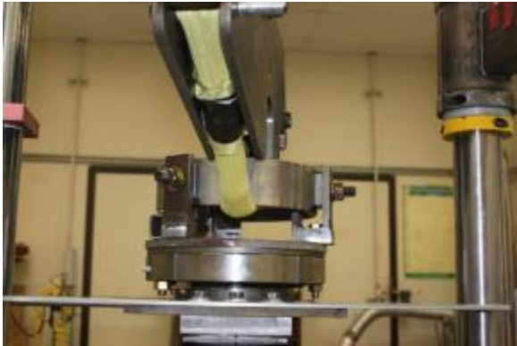
Photo 5. Protected riser under load.
