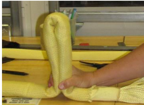
Photo 22. Flexibility demonstration of protected CPAS drogue textile riser.
