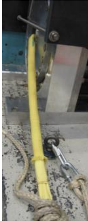
Photo 27. Riser sample at 90° bend angle (Fair Lead analogue).
