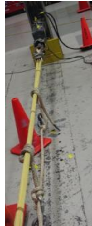
Photo 29. Hydraulic ram and load cell attachment.
