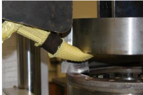
Photo 6. Protected riser under load (close-up view).
