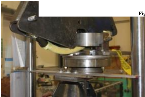
Photo 3. Test fixture with protected riser and contact edge.
