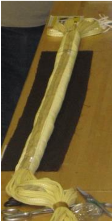
Photo 18. Kevlar cloth inner sleeve secured with Teflon tape.
