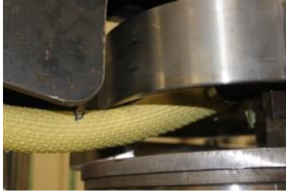
Photo 4. Protected riser and contact edge (close-up view).
