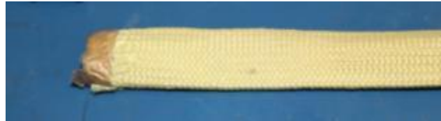
Photo 2. Tubular Kevlar® outer Kevlar sleeve.
