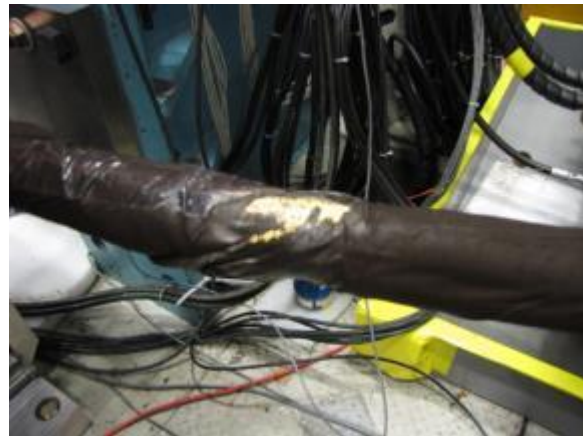
Photo 43. Test 2 effects (Teflon sleeve).
