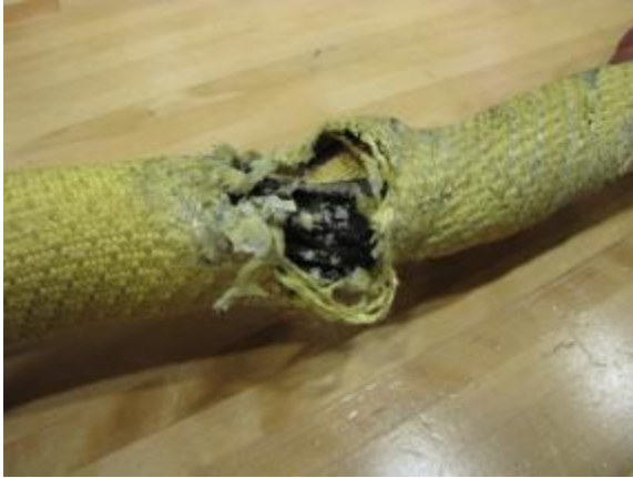
Photo 34. Test 1 effects (outer Kevlar sleeve).
