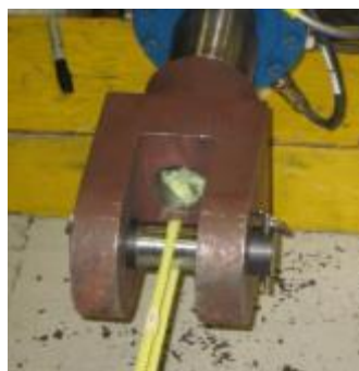
Photo 66. Tensile test fixture (1-3/8" pin).
