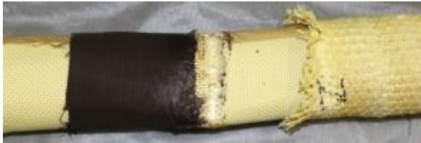
Photo 11. Post-test inner Kevlar sleeve, “N”.
