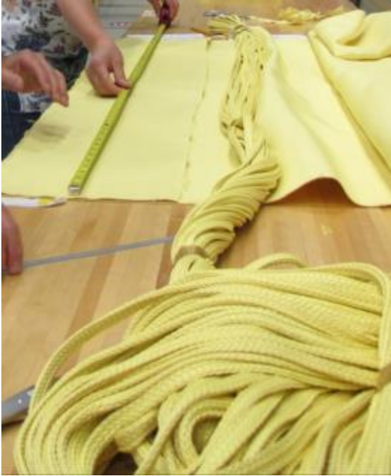
Photo 16. Riser sample about to be wrapped in Kevlar cloth.
