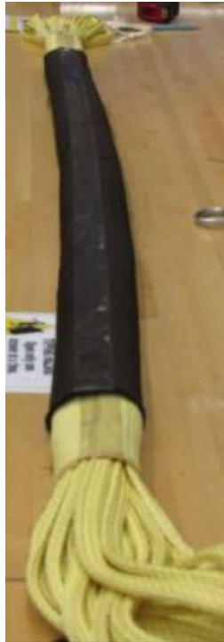
Photo 19. Teflon middle sleeve secured with Teflon tape.
