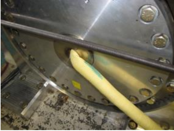
Photo 28. Riser sample in contact with 5/8" edge radius (Fair Lead analogue) and marked to provide visual indication of rotation.
