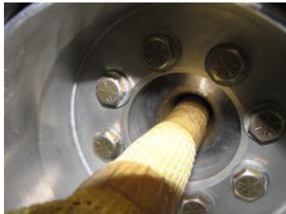
Photo 26. Riser sample passing through edge radius tube.
