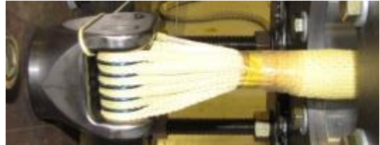
Photo 47. Test 5 taped outer sleeves.
