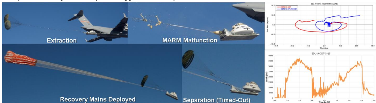
Figure 31: EDU-A-CDT-3-13 Extraction Malfunction at 13,000-ft.
