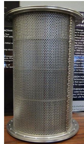
Figure 11. Perforated sheet installed.
