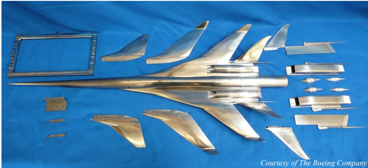
Figure 4-6. Photograph of Performance model and interchangeable parts
