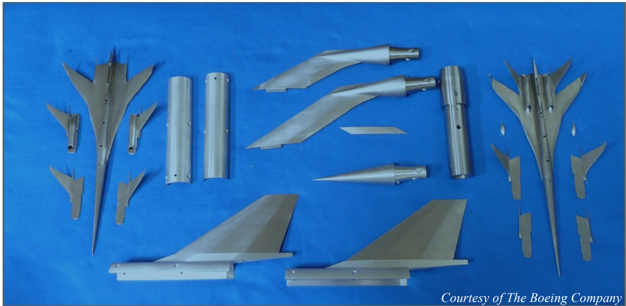
Figure 4–16. Photograph of Boom1 (left) and Boom2 (right) models with interchangeable parts, VS1 and VS2 struts, balance adapter, and adapter fins
