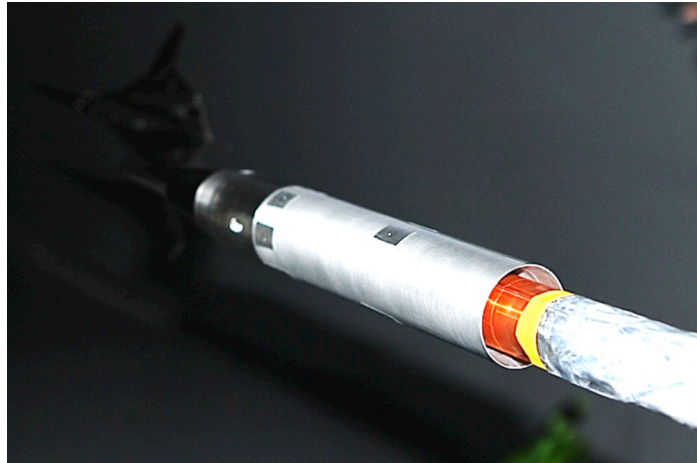
Figure 5–7. Fouling strip, cavity pressure tubes, and thermocouple wires on sting behind balance adapter
