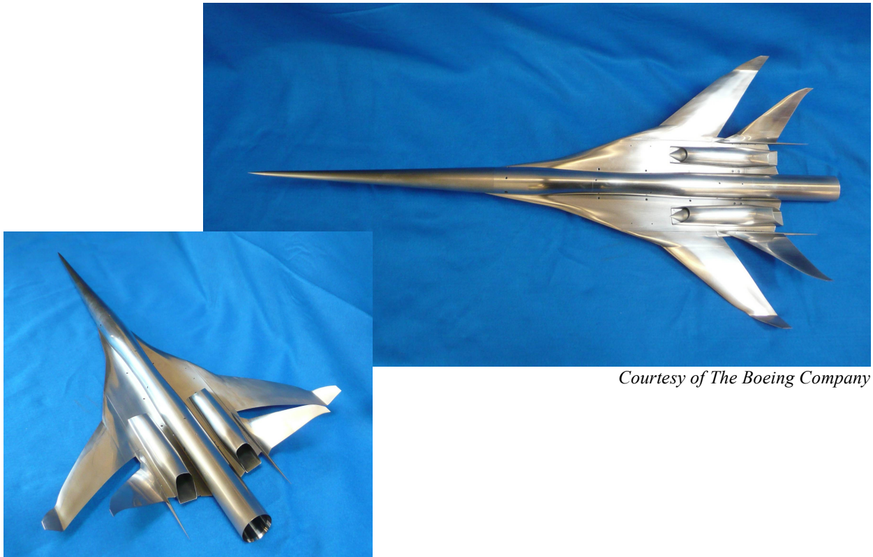
Figure 4-5. Photographs of assembled Performance model with sting can at aft end
