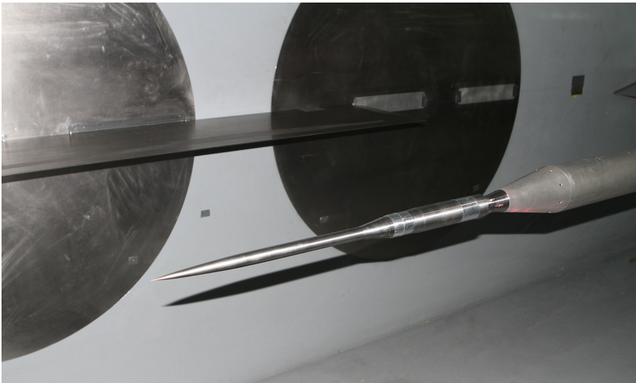
Figure 4–23. Photograph of AS2 model in 9x7 wind tunnel with RF1 rail mounted on forward window blank
