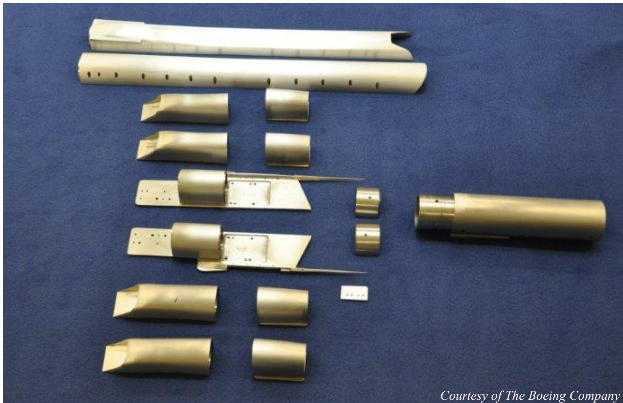
Figure 4-8. Photograph of Performance model new Phase II parts and tailored sting covers
