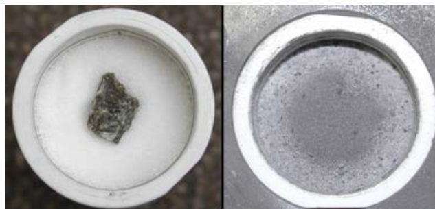
Figure 3.— An enstatite (a form of pyroxene) crystal before (left) and after (right) being pulverized by a ceramic projectile. The inside diameter of the target container is 34 mm (about 1.5 in.)
