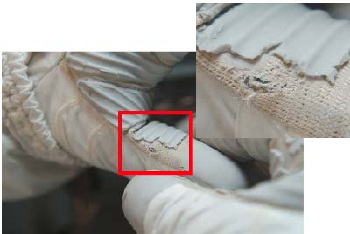
Figure 4.– Damage to the left glove of one of the EVA crew after STS-118 EVA #3.
