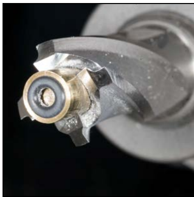
Figure 1.– The coring device developed at JSC. Cores taken have a diameter (measured at the core's painted surface) of approximately 7 mm, corresponding to the inner diameter of the annular cutter.
