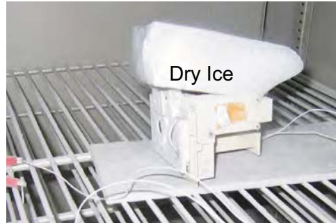
Aperture Cover Mechanism in thermal oven, with N2 purge
