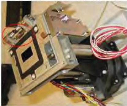
Initial catch design: Bent sheet metal
