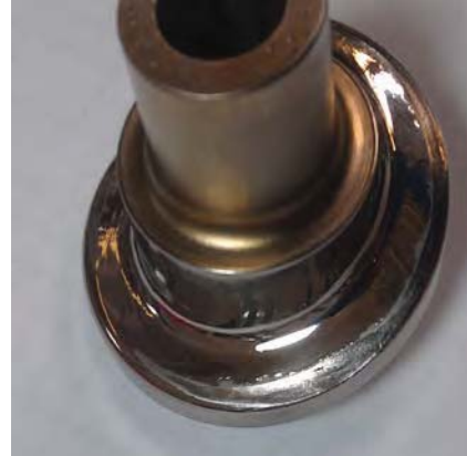
Figure 12. Wear on SASSI CAM
