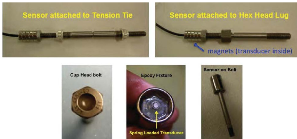
Figure 4. Methods for attaching an ultrasonic transducer to the bolt elements. In the top photographs the magnets are attracted to the nut that is threaded to pull the sensor against the end of the bolt element. The spring-loaded sensor in the bottom photograph is manually pressed against the bolt head.
