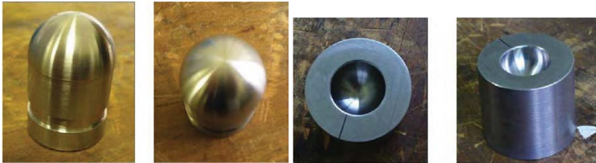
Figure 9. Steel Pin on left and Tungsten cave on right
