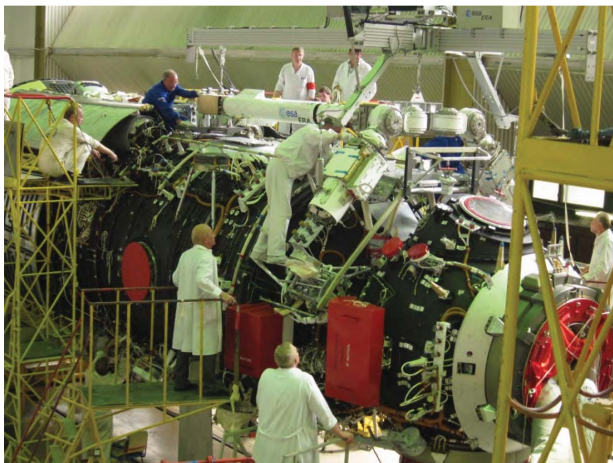
Figure 10. ERA integration fit checks on the MLM
