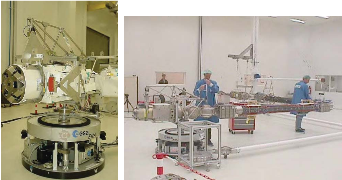
Figure 8. Moving flat floor disc on large flat floor surface (double decoupled)
