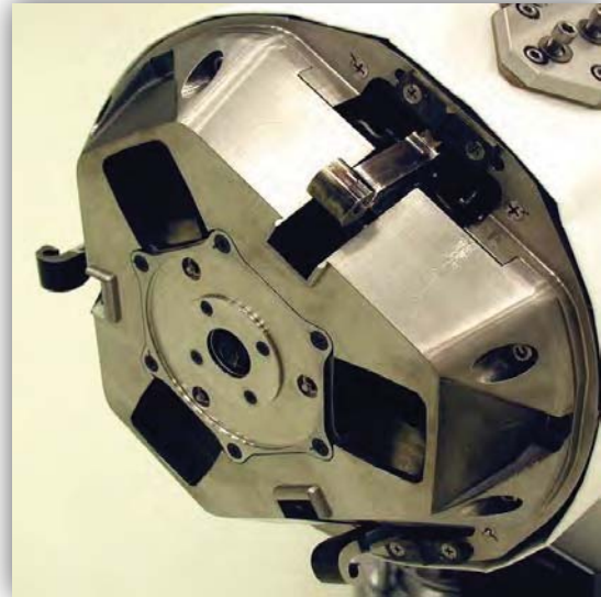
Figure 2. Grapple mechanism with moving table showing the 3 clamps and 3 connectors (retracted)
