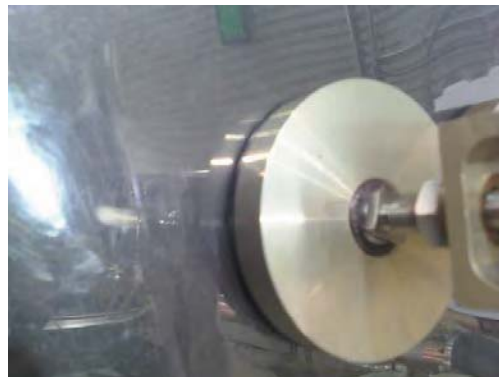
Figure 19. Air Pad Gliding on Melinex 515 and Poron 4701-30
