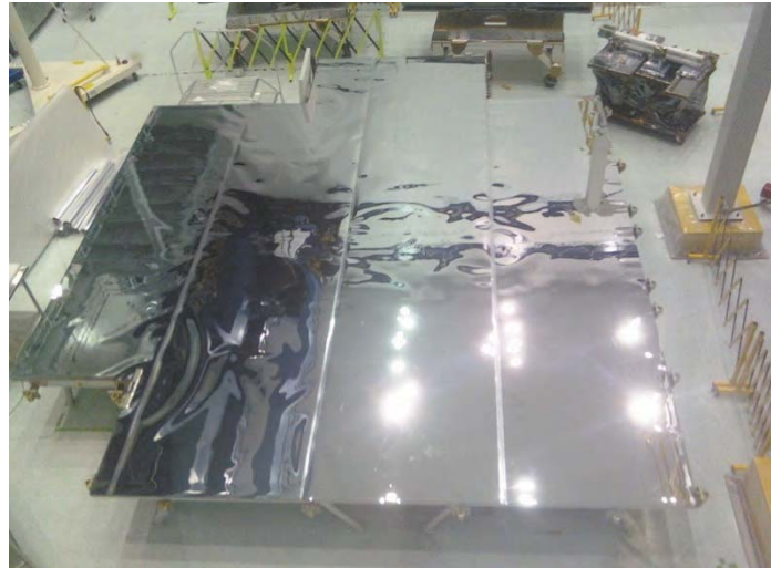
Figure 21. G-negation Table with Melinex 515 and Poron 4701-30
