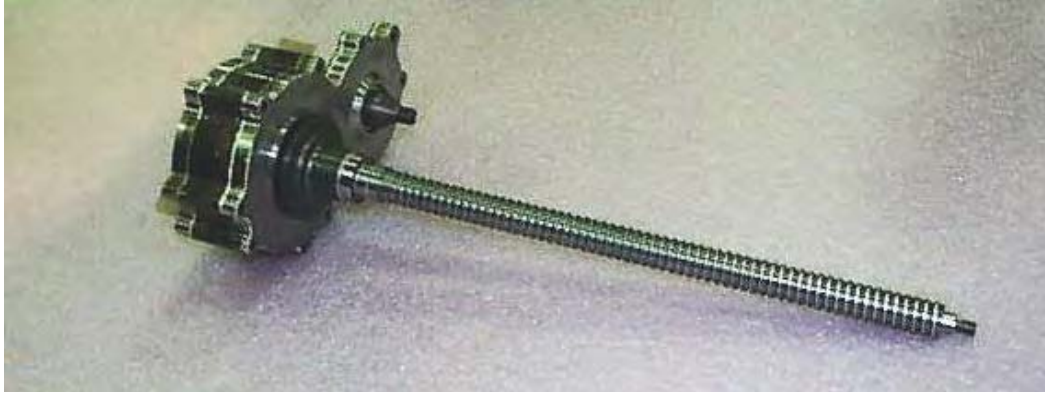
Figure 4. SSRMS LEE Rigidized Gearbox With Ballscrew, Scale: ballscrew = 18-in long (46 cm) (Courtesy of MDA Corp)
