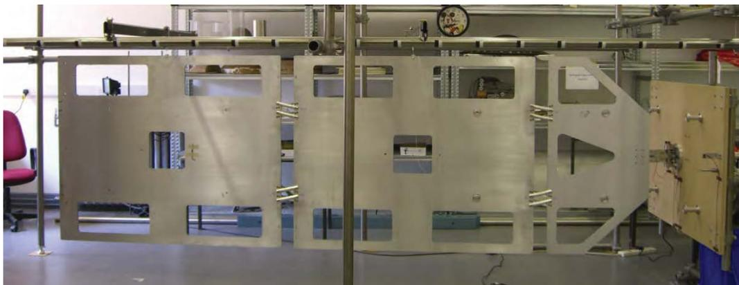
**Figure 4. Surrey Rigid Array in deployed position**
