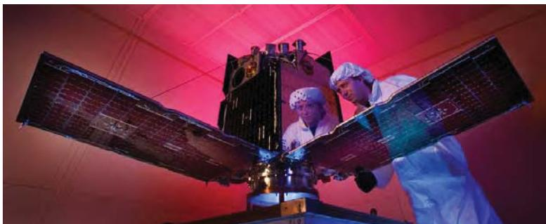
**Figure 1. DMC-CFESAT platform with deployable solar panels partially deployed**
