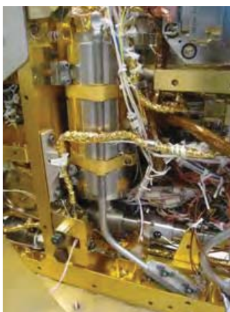
Figure 4. Wide Range Pump Installed in SAM Instrument
